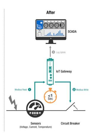
This case illustrates a clear need for an intelligent IoT gateway or an intelligent edge device for faster decision making. A centralized architecture where the data is sent to the Power SCADA for processing does not provide the fast response time that is required.
